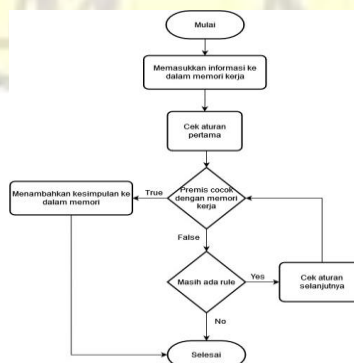
Gambar 2. Algoritma Forward Chaining
