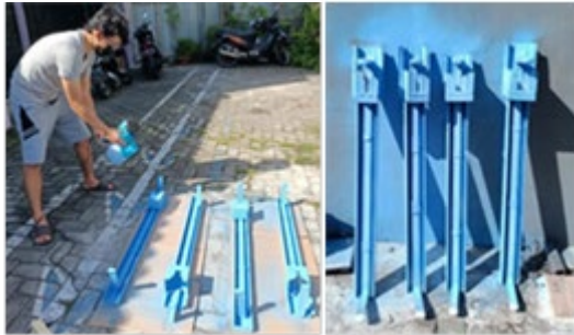
Gambar 2. Pengecatan kerangka hand sanitizer pedal
